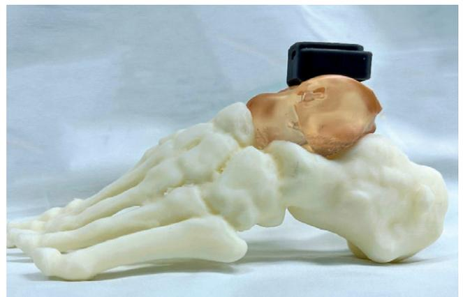
**Figure 2.** Printed talus acrylic template.
